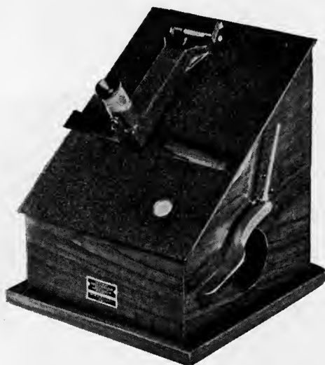
FIG. 3. Eastman direct-reading densitometer; for reading densities on all types of films and plates.
